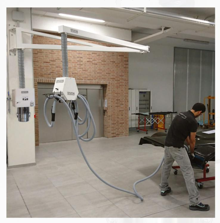
Industrial extractors designed for wall installation, ideal for the connection with an articulated arm. Automatic and manual starter of the single-phase turbine.
