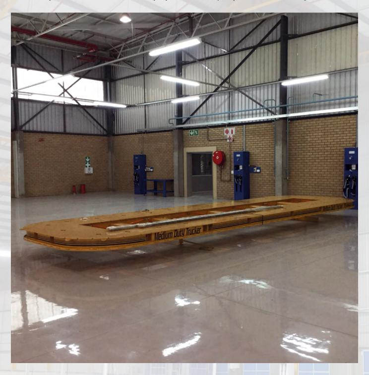
Multipurpose modules for energy distribution: dust extraction, compressed air and electricity. Ideal for preparation zones, it can be used as a built-in module or as a free installation; just connect it and the operator can work immediately.
