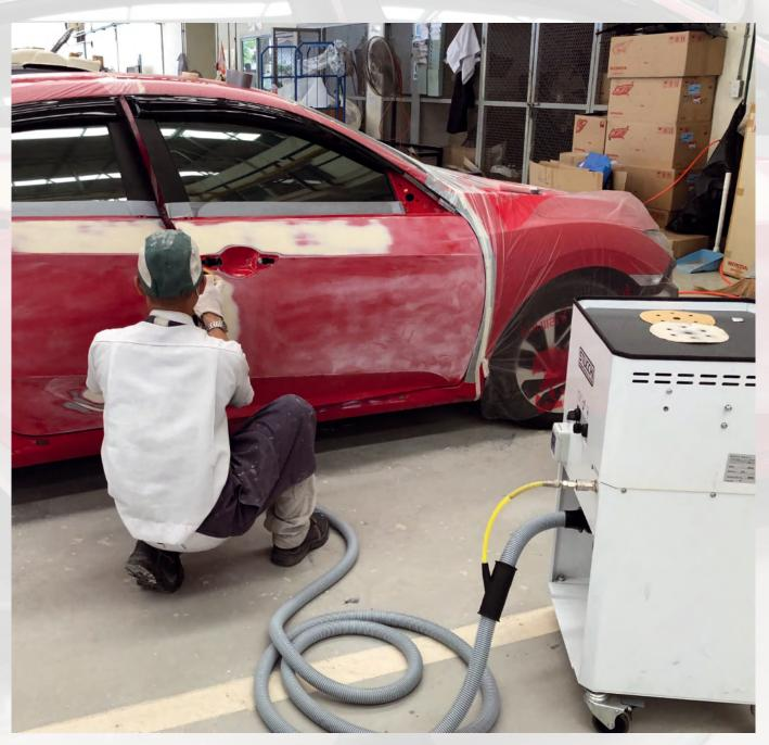
The self-cleaning filter system, unique in its range of reference, is derived from the centralised industrial systems and allows to keep the filters always clean which do not require any maintenance. The use of a tool automatically starts the suction turbine that will turn off when you stop working, thus reducing fuel consumption.
