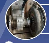
Borg & Beck CSC's are quality controlled on our CSC test rig, putting them through 100,000 cycles at 140° to replicate the on vehicle operating temperatures.
