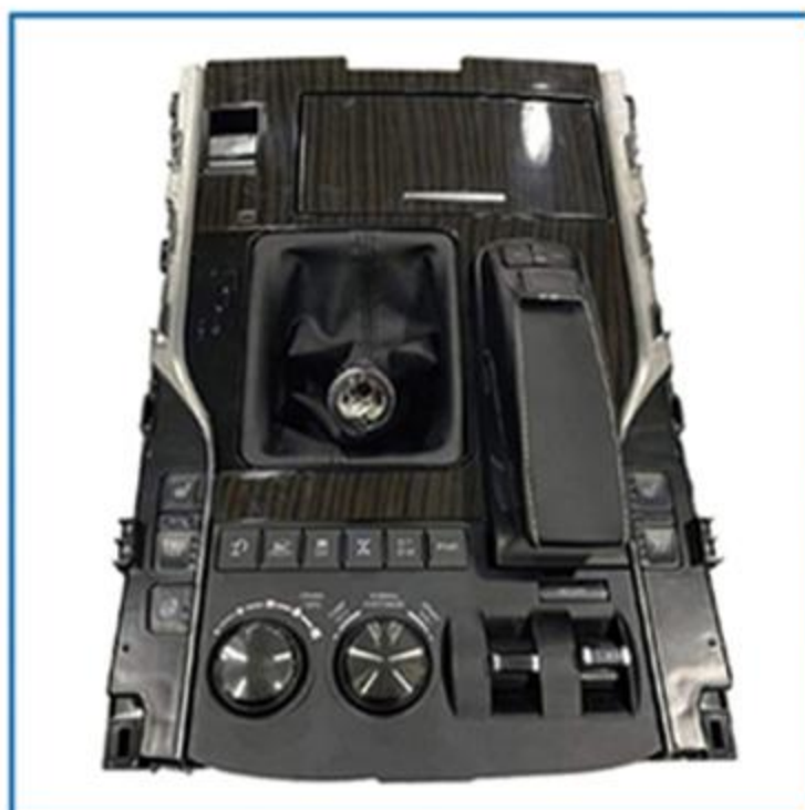
32.Crawl switch assembly
