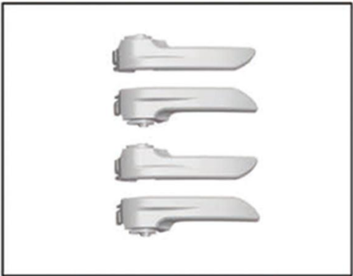
Integrated modified inner handle
