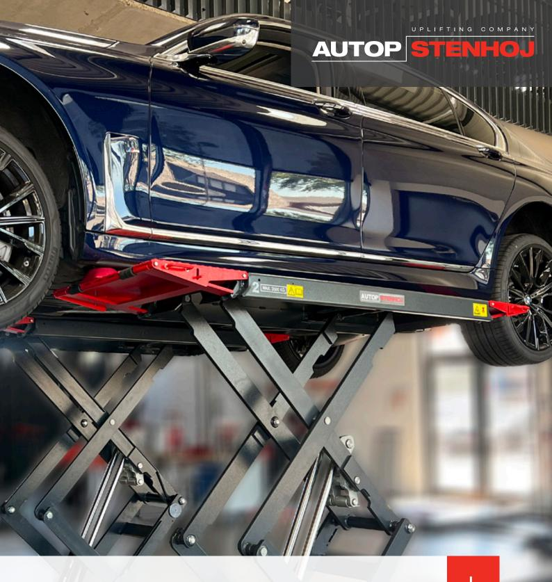
Electro-hydraulic double scissor lift with 3.5 t capacity
