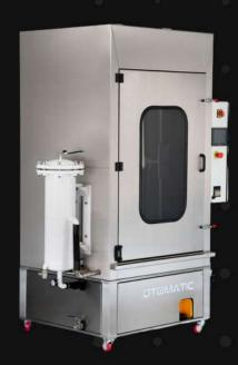
In both machine models, the operator has the option to install the DPF filter for cleaning in the machine cabin using a pneumatic actuator equipped with a rubber sleeve, operated by a foot pedal, or through the use of individual connecting adapters.
