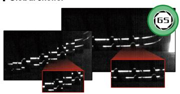
All pixels of the array are exposed simultaneouslyideal for fast moving events.
