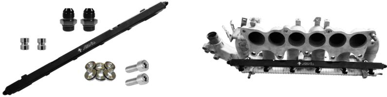
Our Nissan RB25 fuel rail is designed to convert the old side feed set-up found in the RB25DET engine to top feed. This fitment can support our ASNU injectors from 300cc up to 1500cc in our standard fitments.
