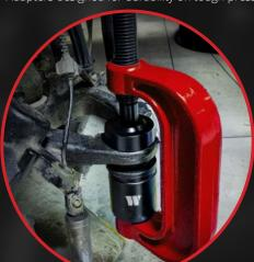
Removes and installs **U-JOINTS BALL JOINTS**
