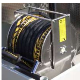
Hose reel equipped with rollers
