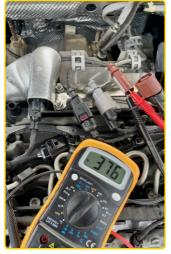
multimeter. If the sensor is installed in an invisible area, it helps to compare the cable colours on the plug connections with the existing circuit diagrams, as the different sensors are usually connected with different coloured cables. If a fault is detected, the sensor must then be exposed and visually inspected.
