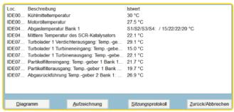
When HC and CO oxidize, heat is generated. As a result, the exhaust gas temperature increases significantly after the catalytic converter. If a temperature is detected that is too low due to a defect in the rear sensor, there will be a deviation from the specified reference values. As a result, the
