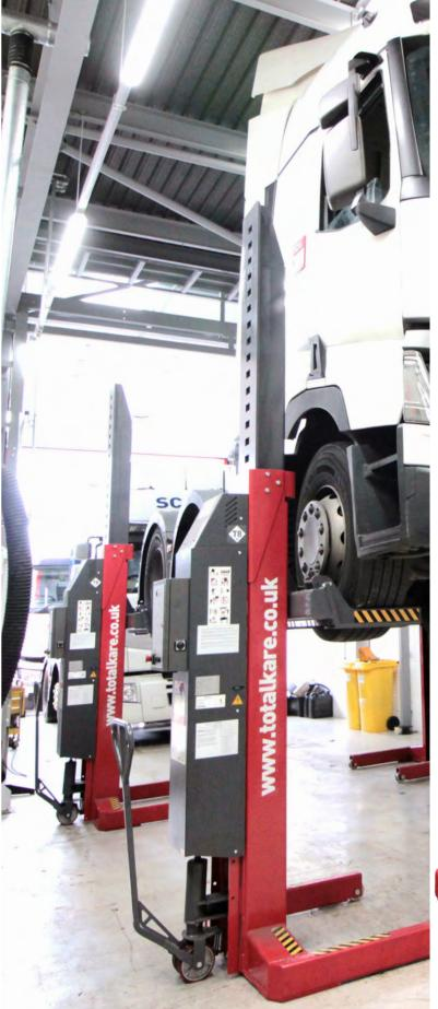
The T8DC cable-free mobile column lift is a versatile lifting solution, with each column capable of lifting up to 7,500kg.
