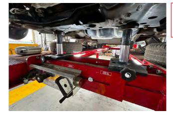
Jacking beams are a vital piece of equipment for vehicle lifts and pits, allowing you to lift vehicles to gain access to key components on vehicles whilst on the vehicle lift. The heavy duty commercial jacking beams from Totalkare are available in 12,000kg, 16,000kg and 20,000kg lifting capacities.
