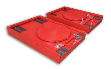
Vehicle radius plates allow the technician to turn the wheels of a vehicle in a desired direction mechanically, without using the steering wheel inside the vehicle.
