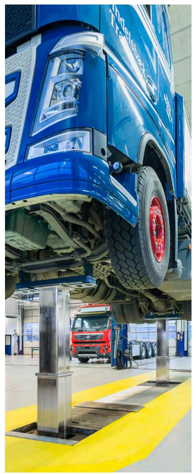
With the primary use of a vehicle lift being to work underneath and around the vehicle, an in-ground lift provides more clearance to a technician wanting to get to all parts or the vehicle, with limited obstruction.
