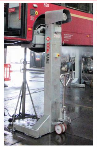
A flexible, cost effective solution for outdoor applications where a permanent lifting location is not required, the G8AC washbay mobile column lift is a truly versatile solution for heavy duty commercial workshops
