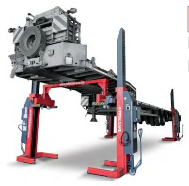
Increase your working flexibility with our trailer beam, which works in conjunction with mobile column lifts to enable trailers to be lifted without the tractor unit.
