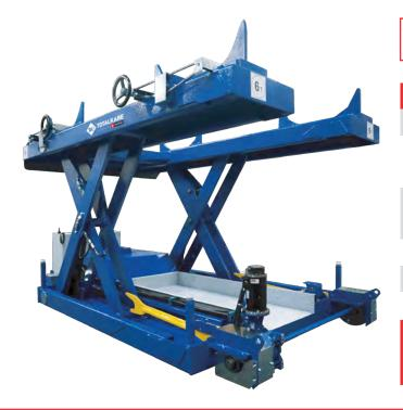
The hydraulic bogie lifting platform which runs on rails, allows the handling, removal and the assemble of railway bogies during maintenance.
