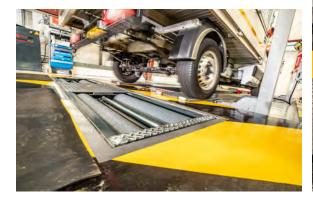
Our DVSA-approved Class 7 in-ground brake tester is strong, durable and suitable for testing all vehicles up to a maximum axle load of 6,000kg.
