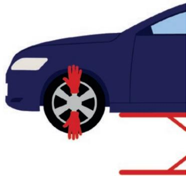
Checking for play on the wheel bearing
