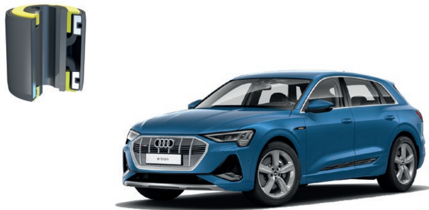
The Audi e-tron's track control arms are equipped with hydraulic silent blocks. The hydraulic fluid flows through rubber chambers, resulting in better absorption of even the smallest vibrations.
