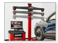
Motorized and manual movable-camera configurations provide a full range of vertical travel for additional lift height.
