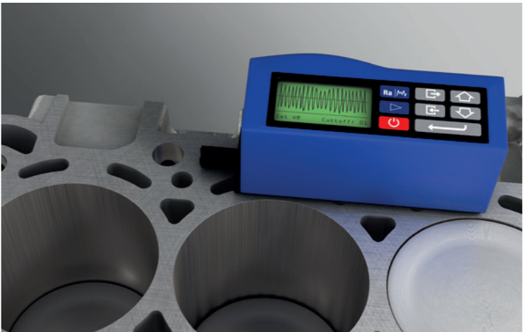
▲ Maximum values for waviness and roughness (grooves and scores) practical measurement using a sensing probe, and indication of possible leakage channels.
