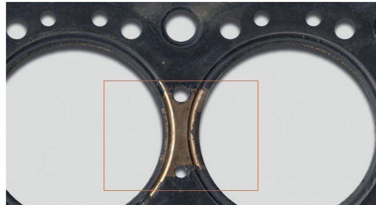
▲ Scorched elastomer coating
