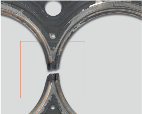
Broken web caused by high component dynamics
