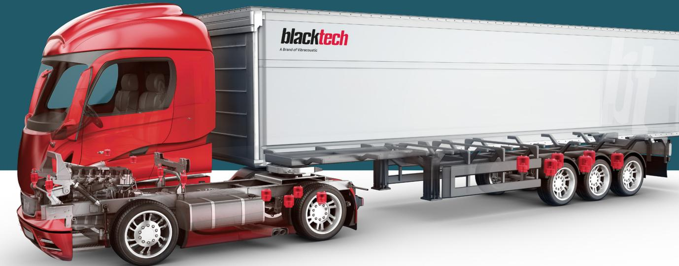
Our broad portfolio of suspension, cabin and seat Air Springs ensures a safe and comfortable ride. From minimum to extreme loads: Our strong quality Air Springs quickly change the spring rate depending on your vehicles' current load situation. blacktech Air Springs provide your Commercial Vehicles a longer cabin and vehicle lifetime along with less downtime and lower operating costs. Improved vibration
