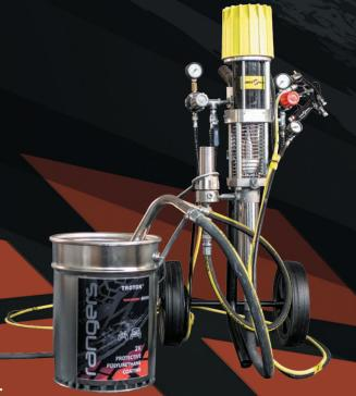
Rangers can be also applied by pneumatic spray using pressure tank and pumps. We recommend to take advantage of this possibility while painting large surfaces.
