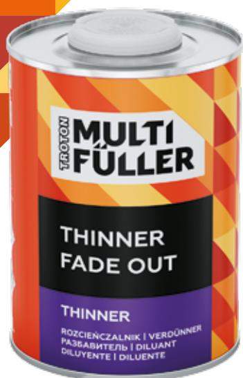
Fade out thinner is ideal for spot repairs on 2 component acrylic clearcoats. Dissolves the dust that settles around the repaired surface, leveling out the optical color difference between the old coating and the newly painted one. Guarantees easy and fast shading, also when using high-solids (HS and UHS) clear coats.
