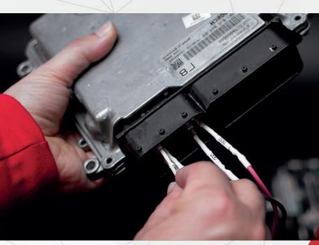
**FLEXBOX:** facilitates mechatronic workflows with safe and immediate bench **connections.**
