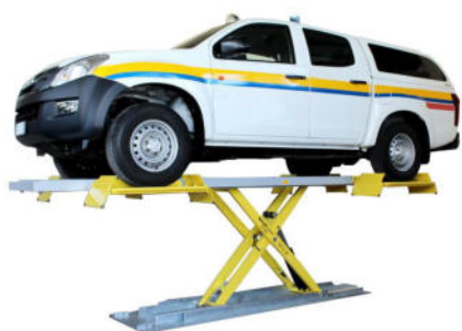
Standard lifting by wheel lifting supports
