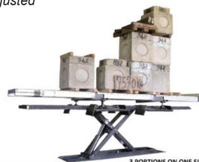
LOAD TEST ON RUBBER BLOCKS AND + 50% OVERLOAD EN 1493 EUROPEAN STANDARD 3 PORTIONS ON ONE SIDE 1 PORTION ON THE OPPOSITE SIDE
