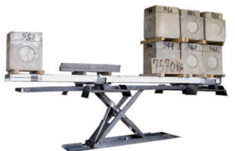
LOAD TEST ON WHEELS + 50% OVERLOAD EN 1493 EUROPEAN STANDARD
