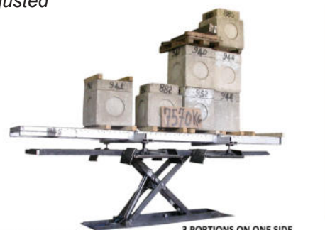
LOAD TEST ON RUBBER BLOCKS AND + 50% OVERLOAD EN 1493 EUROPEAN STANDARD
