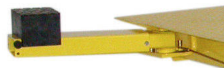
The telescopic lifting arms are inside the footprint area of the vehicle that has been raised, for the safety of people working near the vehicle
