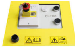
Emergency stop button with lock against non-authorized use
