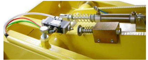
Safety device stopping the lift when exiting the pit, against damage to the underside of a vehicle, and before entering the pit
