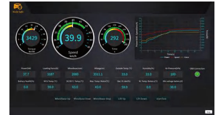
Electric Vehicle Discharging Dyno Interface
