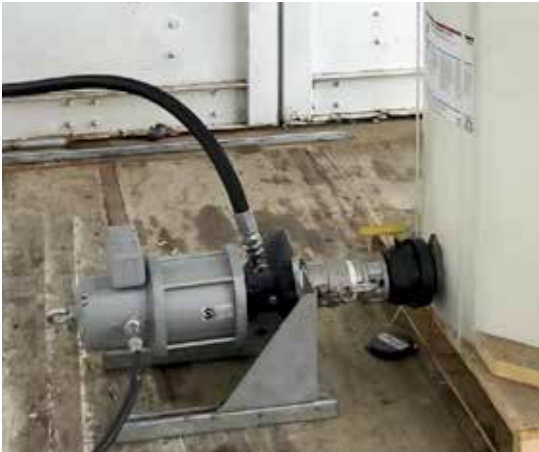
Tank horizontal mounted pump kit for massive grease transfer.
