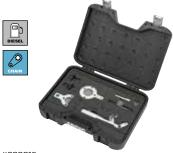
Engine timing & rebuild set Fiat, Opel, Ford, PSA jtd diesel - 1.3  $829016\,\mathrm{has}$  been developed to allow the user to change the cam chain on the later 1.3 jtd/cdti & hdi diesel engines
