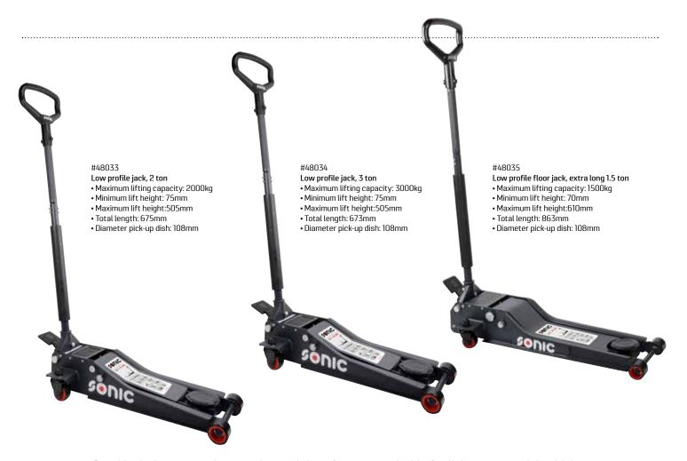
Steel jacks in an extra low version and therefore very suitable for light commercial vehicles. The jacks are equipped with nylon wheels (2 swivel wheels) and an extra foot control. Furthermore, the jacks have a two-part operating rod with handle and a protective foam cover. The jacks come with a pick-up dish with a rubber pad and an extra shell for small material.
