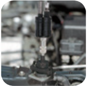
Pressure testing by hand pump.
