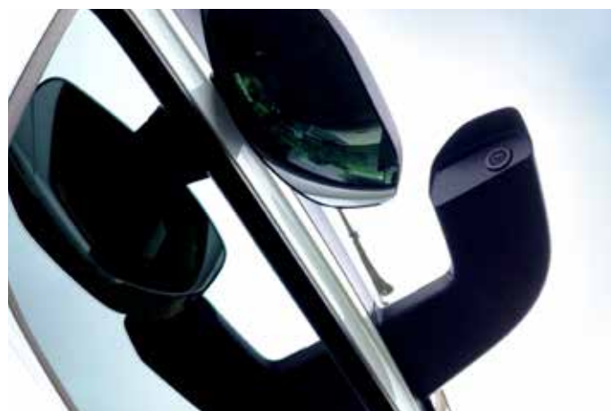
MirrorCam on the vehicle exterior
