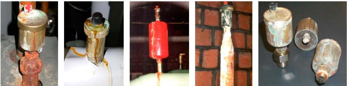
Example of poor-quality air vents, which soon begin to leak due to their faulty construction
