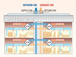
The air quality in a building is one of the main factors for internal comfort. The air must be continuously changed to maintain safe conditions. This process wastes energy, which can be recovered by installing a plate heat exchanger. Let's examine a drugstore with an area of 1235 m², and an average density of 310 people. To change the air, 10,000 m³/h of fresh air, is needed. The example shows a system with our air to air plate heat exchanger:
