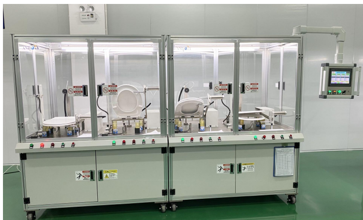
DIN Standard Forced Close + Slow Close Test
