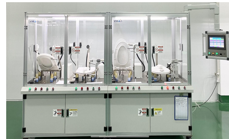
NF Standard Forced Close + Slow Close Test
