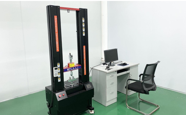
Damper Pull Test
