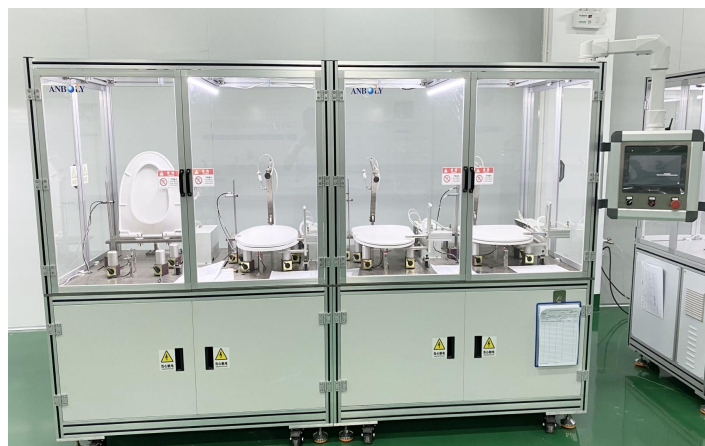
Insert + Pull Lifetime Test
