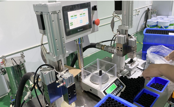
Intelligent Weight Control of Damper Grease
