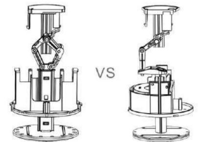
Central lift technology vs Traditional mechanism lift
