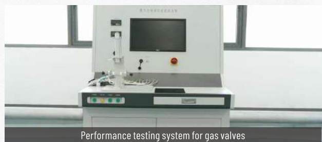
Gas valve leak-tightness performance testing system
