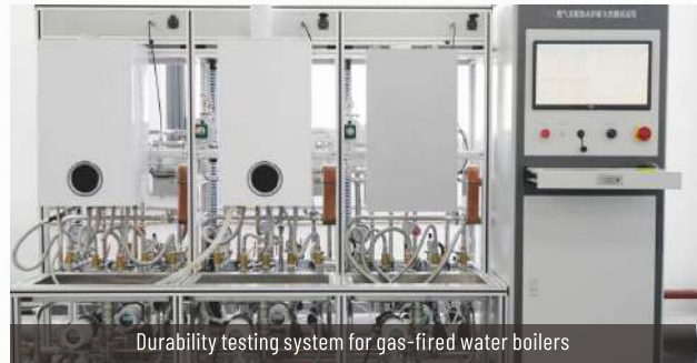
Comprehensive performance testing system for gas-fired water boilers
