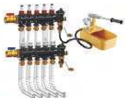
连接系统测试泵至末端配件的填充， 将整个回路加压至最大8bar的压力 Connect the system test pump to the filling valve of the end fitting. Pressurize the entire circuit to a pres of up to 8 bar for the specified time.
