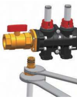
固定好适配器和管道配件 Fix the adapter and pipe fittings.
