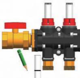
在管道末尾做个标记 Make a mark at the end of the pipe
