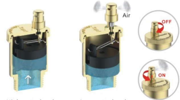
High water level no exhaust Low water level automatic exhaust
