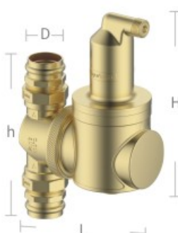
Air Separator with Swivel Connection Material: Brass forging Inside: T2 copper spiral mesh Removed microbubble: \geq 10\mu\text{m} Installation: 360° no dead angle Medium: water, water/glycol(1:1)
