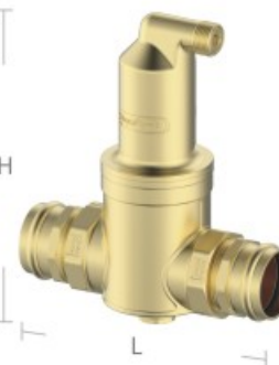
Air Separator Material: Brass forging Inside: T2 copper spiral mesh Removed microbubble: \geq 10\mu\text{m} Installation: Horizontal Medium: water, water/glycol(1:1)
