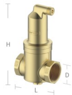
Air Separator Material: Brass forging Inside: T2 copper spiral mesh Removed microbubble: \geq 10\mu\text{m} Installation: Horizontal Medium: water, water/glycol(1:1)
