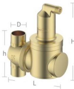
Air Separator with Swivel Connection Material: Brass forging Inside: T2 copper spiral mesh Removed microbubble: \geq 10\mu\text{m} Installation: 360° no dead angle Medium: water, water/glycol(1:1)
