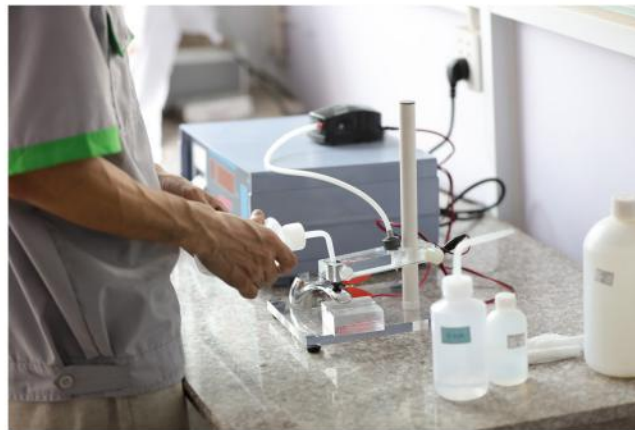
电镀的镍、铬测试 Machine for chrome (Ni & Cr) test
