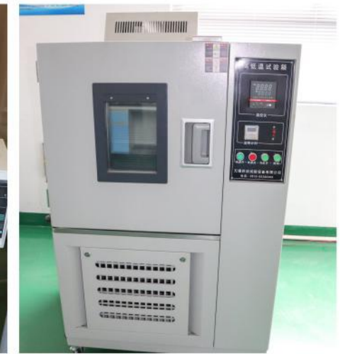
高低温试验箱 High and low temperature test machine
