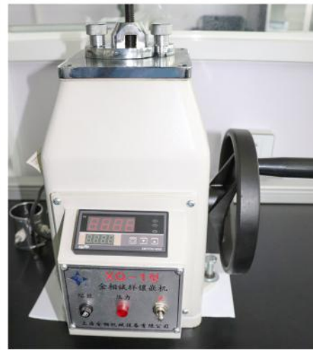
金相试样镶嵌机 Metallographic sample mosaic machine
