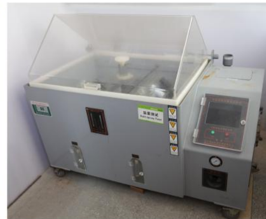
盐雾测试 Machine for salt spray test
