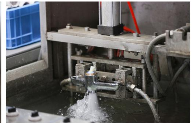
试水机 Machine for water test
