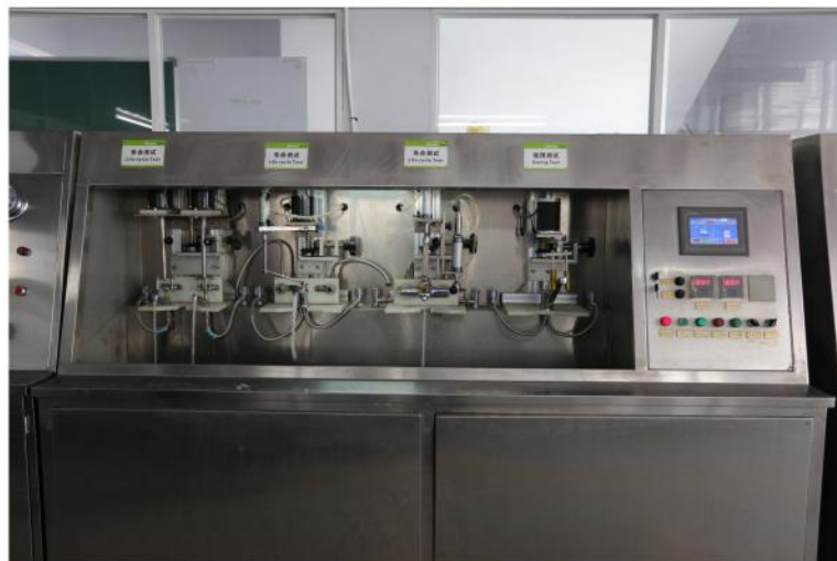
阀芯寿命，提拉，摇摆测试 Machine for cartridge/diverter/sway test
