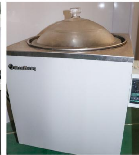
氨熏测试机 Ammonia fumigation test machine
