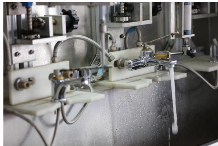
电镀的镍、铬测试 Machine for chrome (Ni & Cr) test
