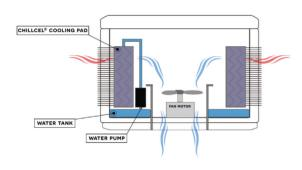
2. As the air blows through the pads water is evaporated and the heat in the air is absorbed
