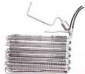
Continuous Fin Type with Heater And Accumulator FF Evaporator
