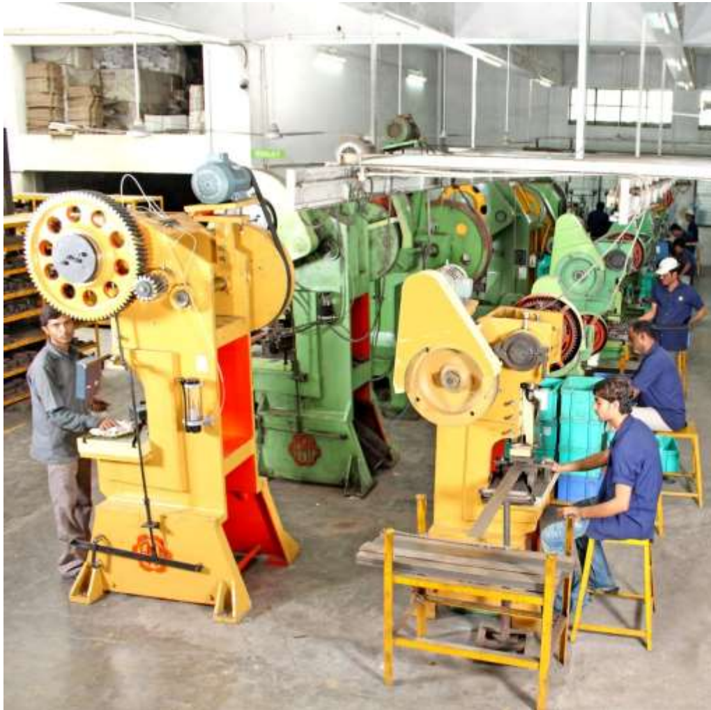
Power Press: 5 ton - 150 ton. (10000 strokes/day)
