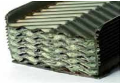
Plate heat exchanger after 6 months in operation: a large part of the paths are calcified – intensive cleaning is necessary.
