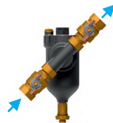
Installing the separator on a sloped pipeline
