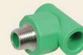
The PP-R overlaps the male brass inserts on the inside. In this way the metal parts are isolated from the installation, and solid deposits and consequently reduced flow are prevented. Moreover, the system is protected against electrochemical corrosion.
