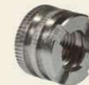
The brass parts (metal inserts) are reinforced, heavy-duty type and of low hardness (105 Brinell) thus eliminating the possibility of cracking, which is particularly common in fittings with female threading. They have cross-shaped grooves at the base of the brass insert so as to prevent torsion and consequent detachment of the metal from the plastic part.
