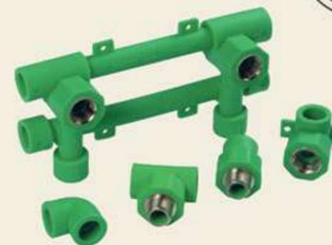
The fittings are manufactured in accordance with DIN 16962 from Polypropylene Random (Type 3) and available in diameters from 20mm up to 450 mm. For the production of the fittings the company uses raw material with a low melt flow index, identical to that of its pipes, so that the mechanical strength of the pipe does not differ from that of the fittings. They are produced with a wall thickness equivalent to 30 bars.
