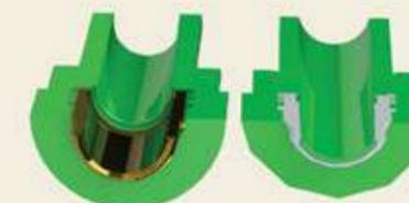
Perimetric fitting retaining grooves, in which one side of the groove has negative declination, from the outside in, so as to retain the PP-R material and prevent detachment of the metal part from the plastic part in the presence of tensile forces.
