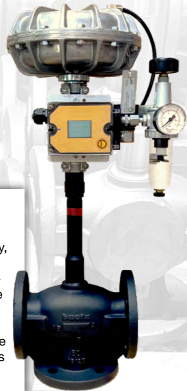
baelz 342-2 with baelz 373-P21 3-way control valve in cast steel. Shown here with cooling tube, pneumatic actuator, I/P positioner and diaphragm pressure regulator
