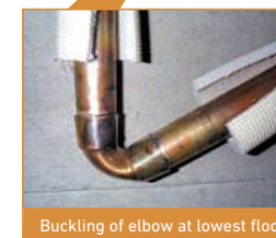
Buckling of elbow at lowest floor
