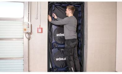
You can easily install one or two devices on windows and doors with our advanced clamp system. If you're missing window or door frames, you can also use an optional installation frame for added convenience.
