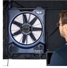
Fully automatic measuring sequence in accordance with DIN EN ISO 9972 or DIN EN 13829 in the entire volume flow range from 15 - 24,000 m<sup>3</sup>/h (with 4 devices) without changing the measuring orifice and overpressure and underpressure measurements without fan conversion.
