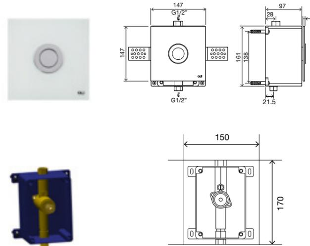
The pre-installation box must be installed before the finished wall phase.
