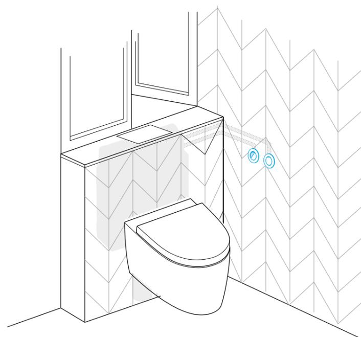
\* Not meant to be used in the opening of the in-wall cistern. An inspection plate (see page 123) should be applied to ensure access to the cistern. Pre-installation necessary.
