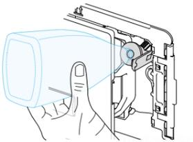
OLIPURE IS A CLOSED STORAGE SYSTEM THAT WITH EACH FLUSH RELEASES A CONTROLLED AMOUNT OF CLEANER INTO THE TOILET.
