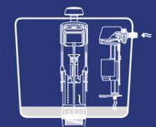
Once the water is flushed, the outlet valve closes and the delaying system makes the inlet valve open to fill the tank.
