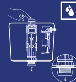
The cistern is emptied faster than the delaying system, while the inlet valve remains closed.
