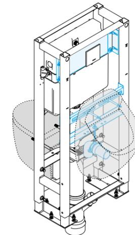
Independently of the bathroom, this product allows to place in one side a toilet and on the other side, a urinal or a washbasin, according to the acquisition of the kits and by sharing the same waste pipe connection, thanks to the evacuation pipe in Y shape. It is prepared to be fix to the floor suitable for plasterboard wall in technical frame.
