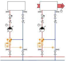
Supply temperature control (weather-compensated)
