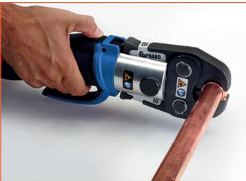
6) Set the pressing tool properly and make sure that the toroidal chamber is inside the jaws. Carry out the pressing until the jaws touch each other.
