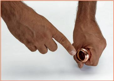
3) **Check the correct position of the O-ring** inside the toroidal chamber and lubricate it with water and soap. Do not use oil or grease at all.
