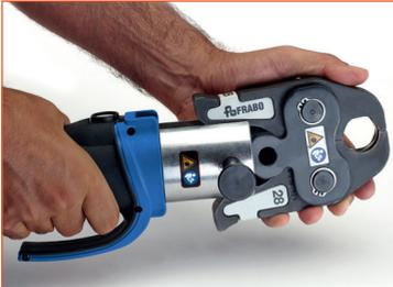
5) Provide the pressing tool with the suitable jaw (V) corresponding to the diameter of the fitting to be pressed.
