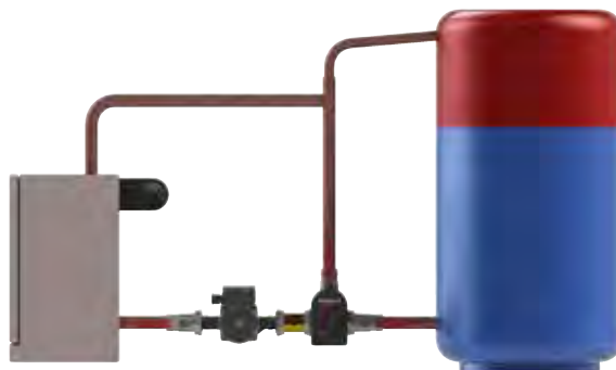
Example showing Thermomatic TVM installed for control of the return temperature to the boiler, Laddomatic.
