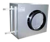
Duct type heating/cooling coils are assembled in cabin as suitable to mount inside duct and have standard capacity. Coils consist of copper tubes and aluminum fins. Inlets and outlets of cabin are suitable for circular duct connections as in heat recovery ventilation units. Additionally, cooling coils have drain pan and extra insulation to prevent condensation of cabin.
