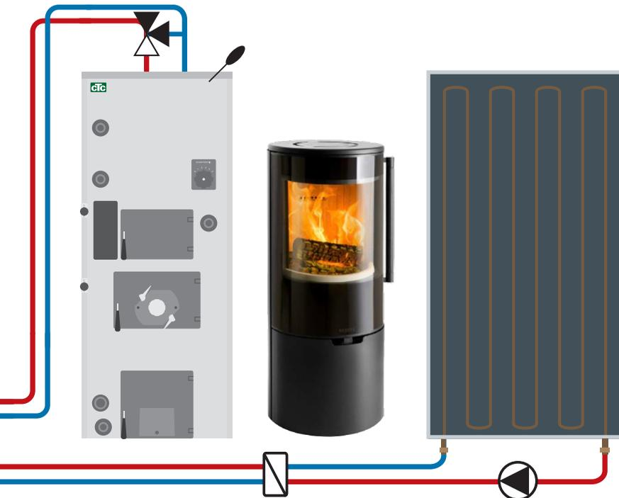
With various smart EnergyFlex accessories, you can connect and control external heat sources such as water-jacketed stoves, solar collectors and wood, pellet, oil or gas boilers.
