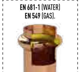
The fittings EFFEBI PRESS "UNICO" are in Copper Cu DHP 99,9 and are usable for both WATER and GAS. The marking on the fittings ( Gas in yellow and water in blue ) are clearly showing this universal range. The O'Ring is conform to the EU norms EN 549 e EN 681/1. The threaded press fittings are manufactured in bronze CC499k.
